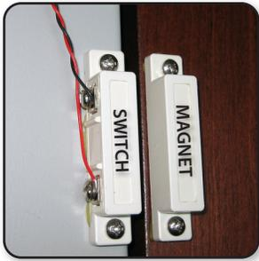
You probably know how a reed switch works. Two springy nickel-iron blades sealed in a hermetic capsule are attracted together when a magnet approaches, and when they touch, an electric circuit is completed. The magnet can be an electromagnet or a permanent
